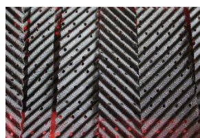
Fig. 3. SS wire mesh strips after catalyst coating and reduction
