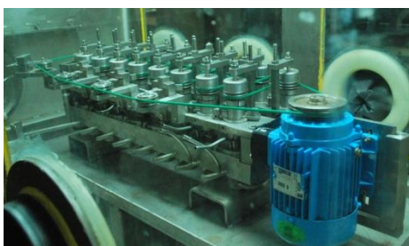
Fig. 1: Photographic view of 16 stages belt driven ACC system
