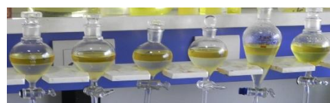
Fig. 2. Settling behavior of TBP (top) and DHOA (bottom) solvents while processing SDU (T)
