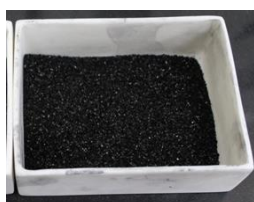
Fig. 1. Carbon Aerogel support synthesized for making Pt-CA powder
