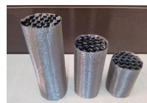
Fig. 4. 3" OD structured packing modules after assembly with heights
